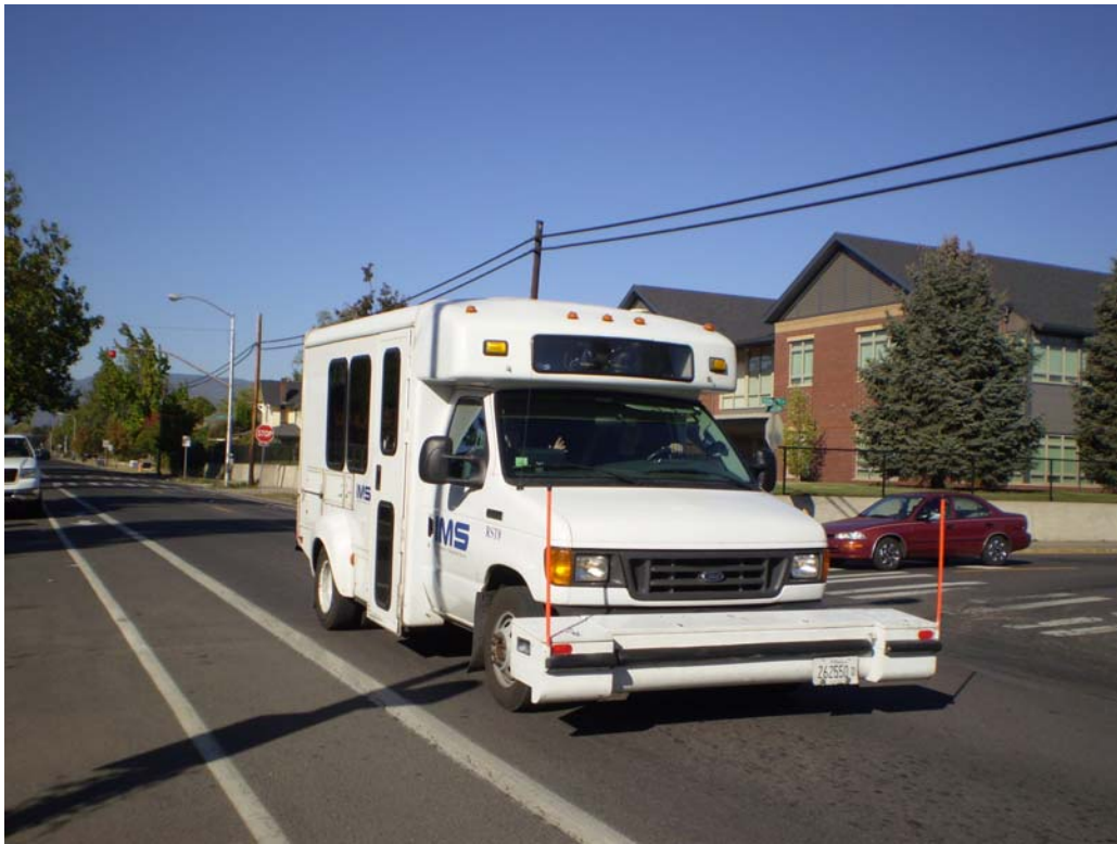
Road surface testing vehicle performing pavement condition assessment on West Jackson Street near Jackson Elementary School. October 2010.
